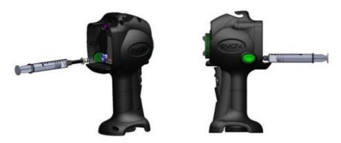
4. Compress the trigger on the spray gun. Point the spray gun at a trash can, sink, backdrop, or somewhere that the liquid can go. While the trigger is pulled, compress the purge tool. Once the water in the purge tool is depleted, detach the purge tool from the spray gun by pushing the green release button and repeat the exercise if this step did not clear out the spray gun.
