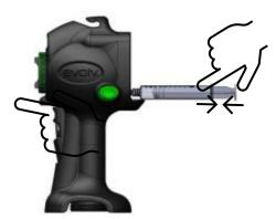
5. If necessary, remove the green air cap retainer, air cap and the fluid nozzle as described in your Owner's Manual and use the Nozzle Tool supplied with your unit. Thoroughly clean all three items with warm water and re-assemble. Also, be sure to clean the fittings located on the back of the spray gun and formulation cartridges.
